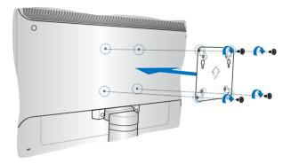
**WARNING!** Do not overtighten the screws as it may cause damage to your VESA mount-compatible device.
